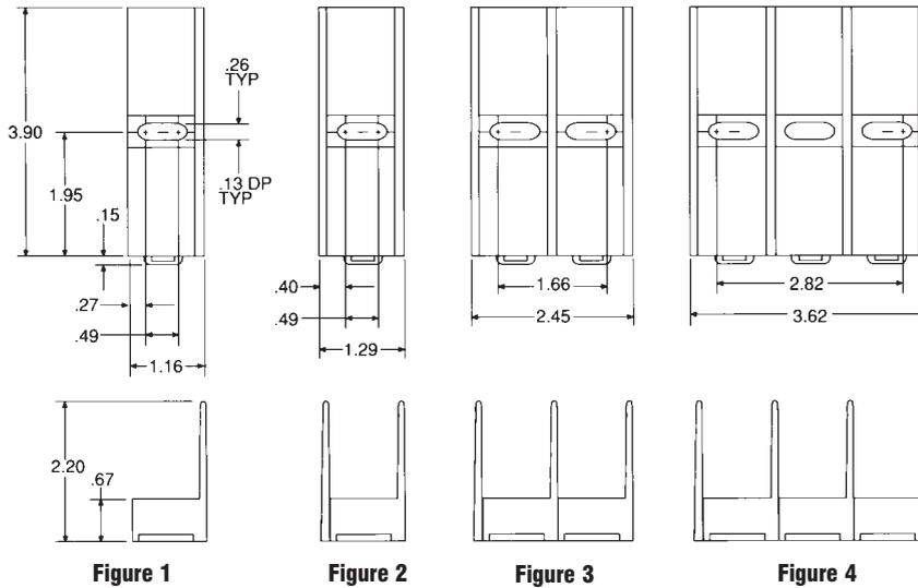
Recommended mounting screws for 30A fuse blocks: 1/4" (.250" dia.)
