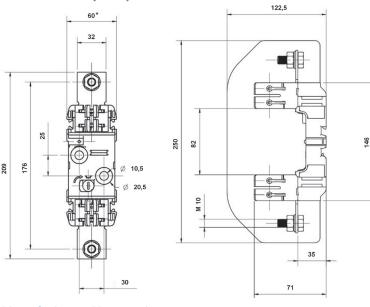
\*86mm for base with protective cover M10 torque recommendation: 230 in-lbs (26Nm)
